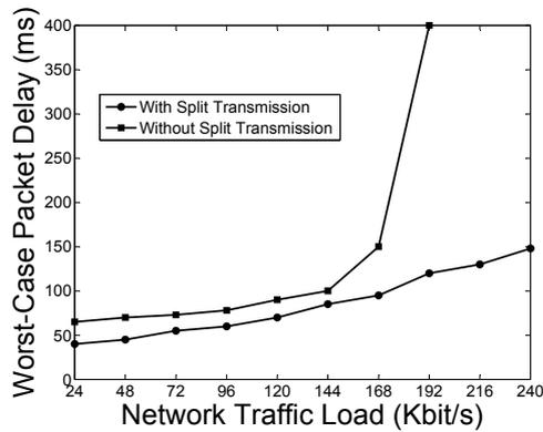
Fig. 7. The worst-case delays in the multiple receiver simulations.
