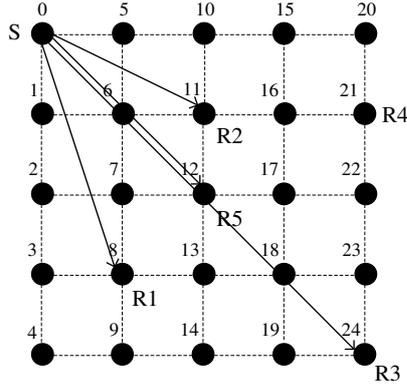
Fig. 6. Network topology for the multiple receiver simulation.
