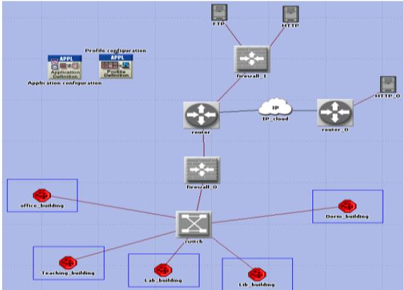
Figure 5 OPNET model for Wired Network
